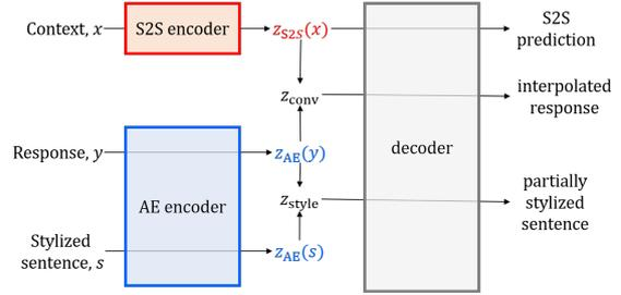
Figure 2: STYLEFUSION model architecture.
