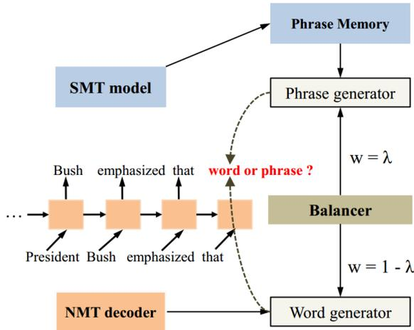
Figure 1: Architecture of the NMT decoder with the phrase memory. The NMT decoder performs phrase generation using the balancer and the phrase memory.
